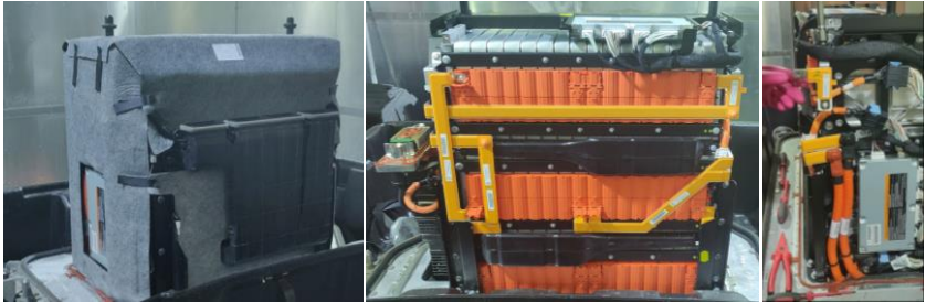
Manual disassembly of the battery pack from the Renault Fluence.*
