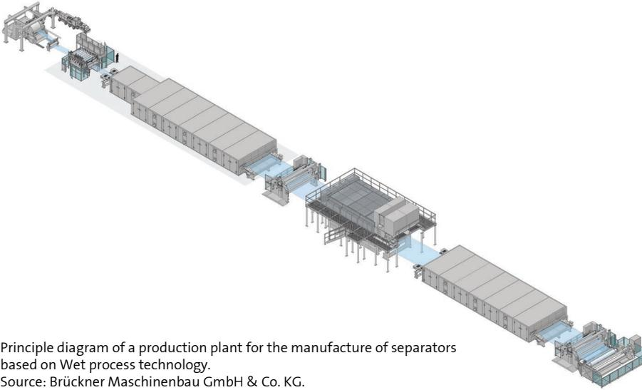
Principle diagram of a production plant for the manufacture of separators based on Wet process technology.
