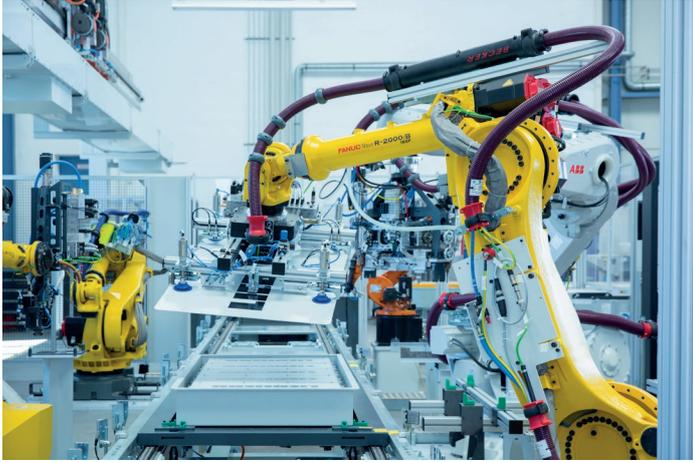
5 modules are assembled to the pack. Picture shows mounting of the upper part of the housing/lid and screwing to the battery pack housing.
