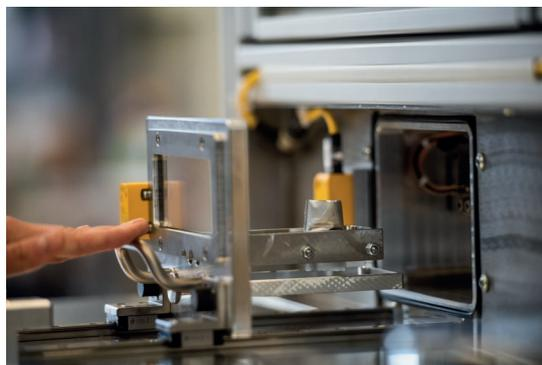
Electrolyte Jet: Semiautomatic electrolyte filling machine for pouch cells with vacuum chamber
