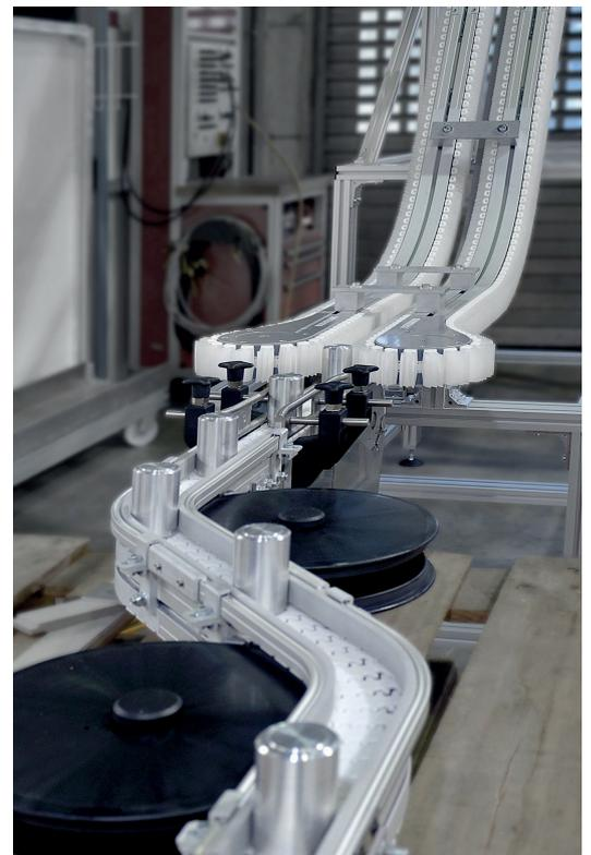
Versaflex conveyor system for the ultra-fast transport of battery round cells in the incoming goods department of an automotive manufacturer - without workpiece carriers, with maximum throughput and high process reliability
