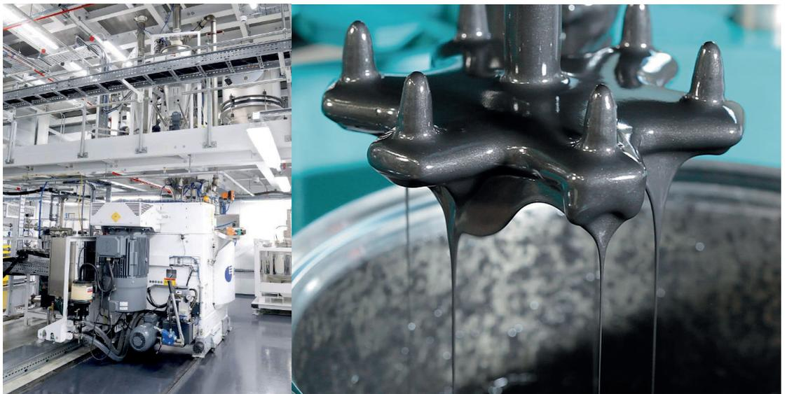
Fully automated 2 GWh mixing plant for coating compounds with Eirich MixSolver® (bottom left) and AZODOS® metering system (top left) at the UK Battery Industrialisation Centre (UKBIC)
