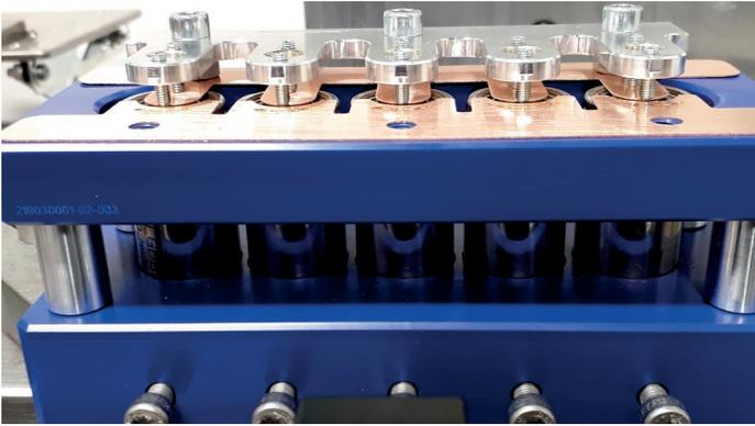
A battery block consisting of cylindrical cells and busbar for the investigation of clamping technology and process parameters in laser welding
