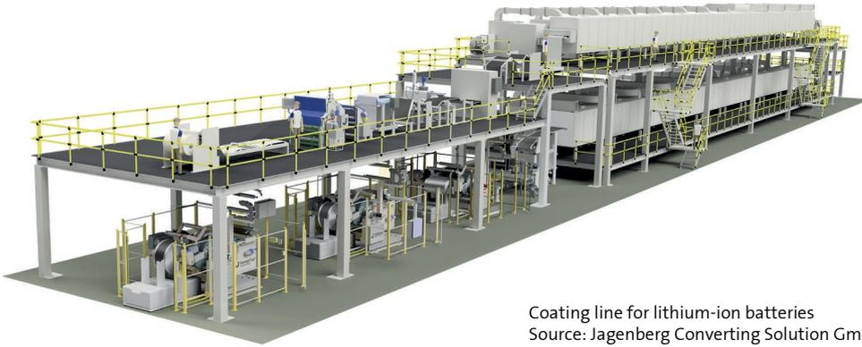
Coating line for lithium-ion batteries
