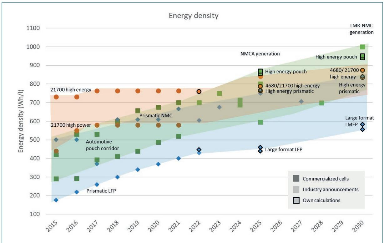
Evolution of volumetric energy density of LIB cells on cell formats [Link2022].
