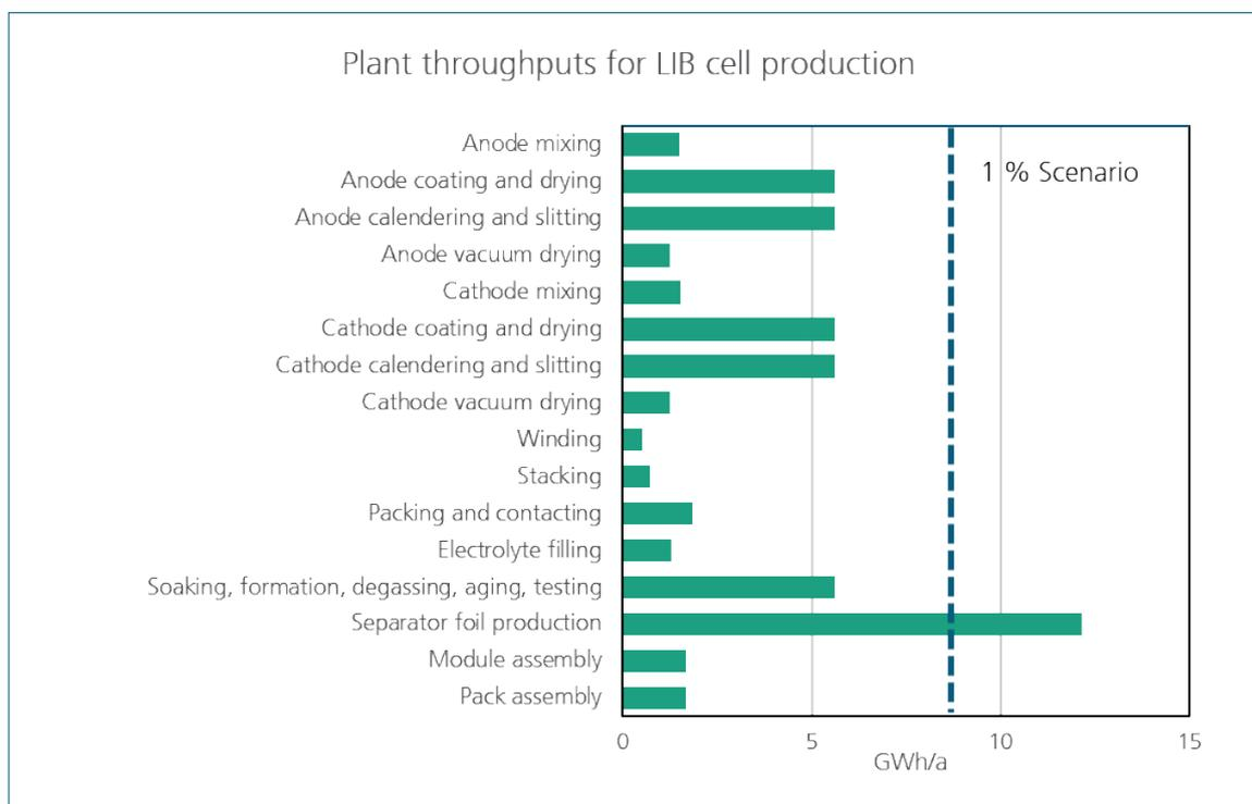
Currently possible plant throughputs of different manufacturing processes (separate anode and cathode production) as well as an illustration of the required throughputs for the one percent scenario.
