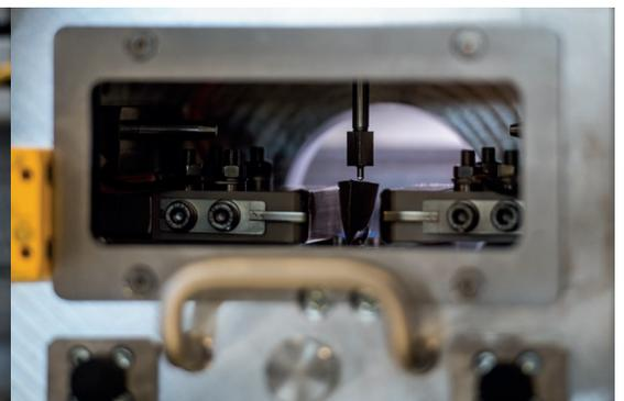
Electrolyte Jet: Precise and fast electrolyte filling system for Li-ion pouch cells
