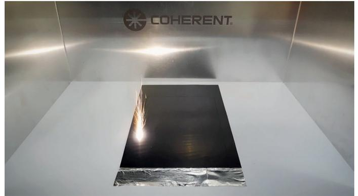
Laser cutting of coated and uncoated electrode material
