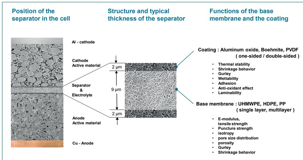
Schematic diagram of a separator typical for EV applications
