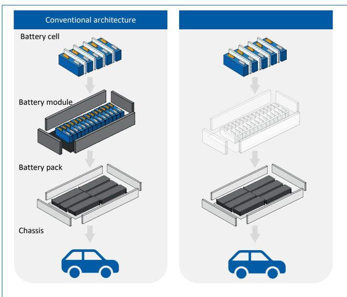
Comparison of conventional system architecture to the cell-to-pack approach
