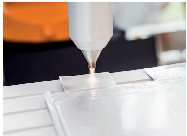
Plasma cleaning of the contact point of a pouch cell
